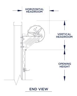
Universal mount 4" deep 12-gauge galvanized steel wind bar guides require no pre-installation modifications for steel, concrete or filled masonry block applications.
