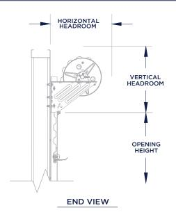
Universal mount 4" deep 12-gauge galvanized steel wind bar guides require no pre-installation modifications for steel, concrete or filled masonry block applications.
